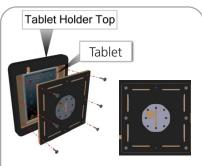
Place tablet into holder. Secure with thumbscrews. Plate on base must be vertical (as shown) to lock properly.
